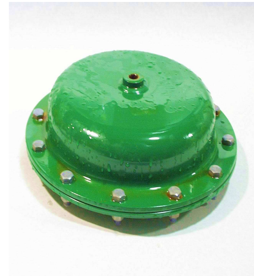
Powder-coated actuator casing with HCF coated cap screws after 500 hours of salt spray
