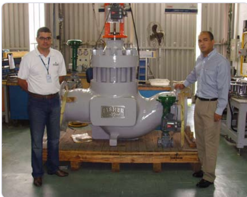
One of the large Fisher valves manufactured in Sorocaba, Brazil, for an offshore oil production platform.
